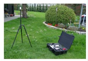
Then the weather station is mounted on top of the tripod, orientated to north and fixed on the tripod with the 2 screws at the socket. Please take care that the tripod stands fixed on the ground to avoid droping of the tripod in case of wind. With internal cabling you may run a laptop in parallell to the measurement.
